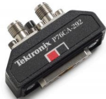
P76CA-292 33 GHz Bandwidth Coaxial Adapter with 2.92 mm (Female) connectors. This adapter is calibrated at the input connectors and is ideal for use with off the shelf or custom cables. Low skew cable pairs should be used to preserve full bandwidth performance.
